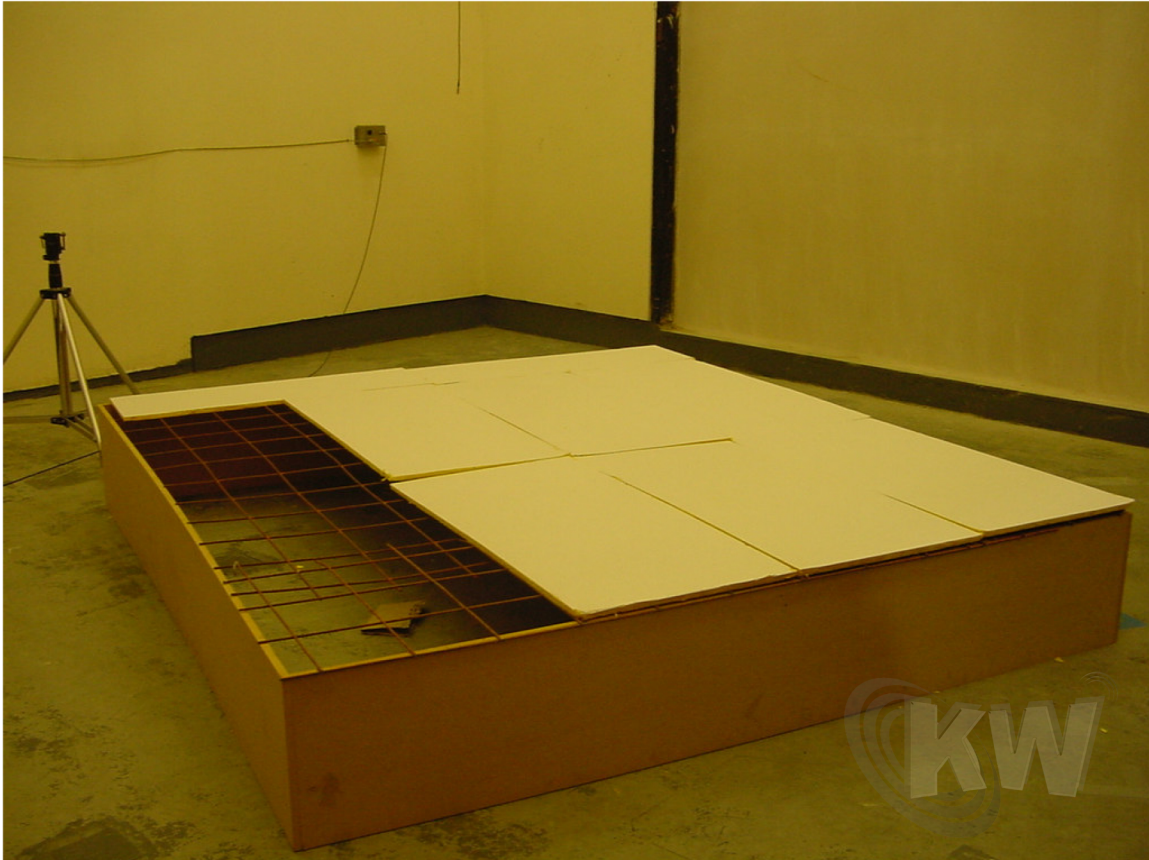
Figure 4.3: Test sample in the process of being fitted to the Type E mounting.
